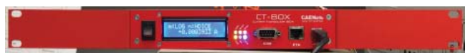
FIG. 1. CAENels CT-Box. The USB cable on the right connects to a PC that runs the CT-Box drivers. The serial cable that allows communication from the CT-150 current transducer to the CT-Box connects to the back.
