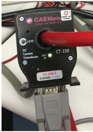
FIG. 5. CAENels CT-150 current transducer. The thick, red cable passing through the current transducer is the high current output lead from the Fluke that forms the current loop.
