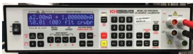
FIG. 3. Krohn-Hite Model 523 Precision DC Source/Calibrator. The cables on the right are the output leads that connect to the Fluke 52120A.
