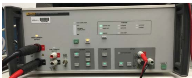
FIG. 4. Fluke 52120A Transconductance Amplifier. The thin, right cables are the input leads from the Krohn-Hite. The thick, left cables carry the amplified high current output.
